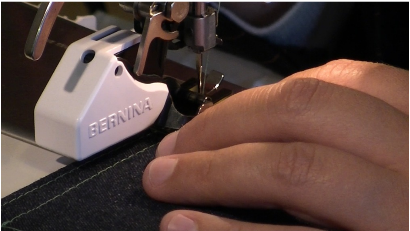
Top stitch with a double row of stitching at the top of the small pocket to secure the rolled seam.
