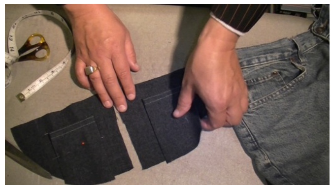
Once pressed, position the small pockets onto the facings and pin into place to secure ready to be sewn onto the facings. Remember to align the left and right pockets so that they look symmetrical for the left and right facings.
