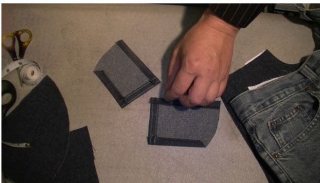
Once top stitched press the sides with a 1 cm seam allowance as shown in the image above.
