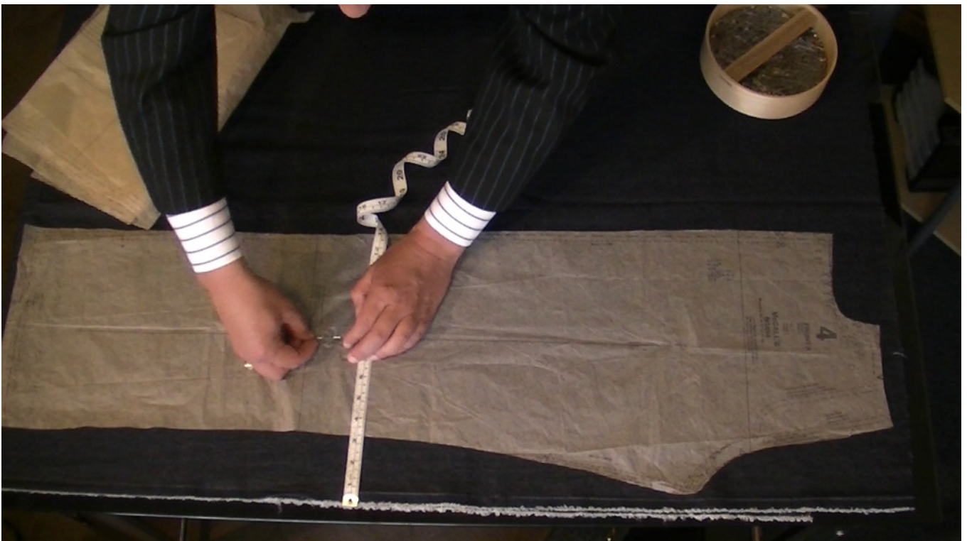
Aligning the pattern pieces onto the fabric by using the grain lines in conjunction with the selvedge.
