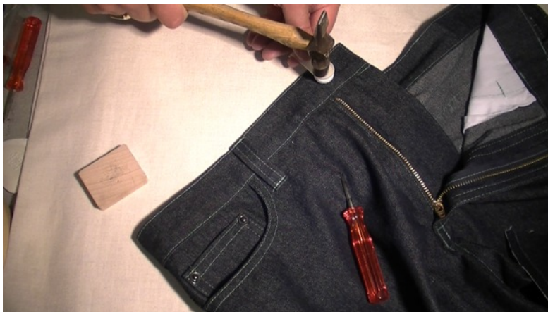
Apply the button in place with a few swift blows of the hammer.
