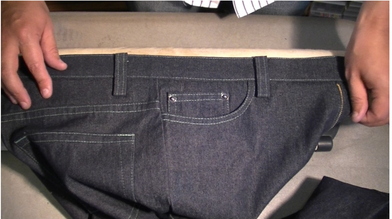
The finished waistband attach to the top of a pair of jeans.
