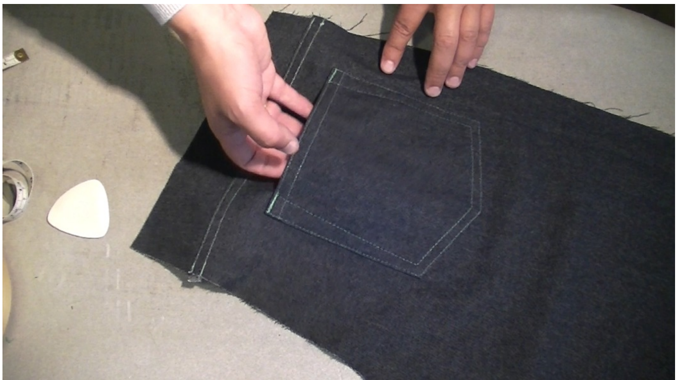
The finished back pockets look decorative with the top stitching in place.
